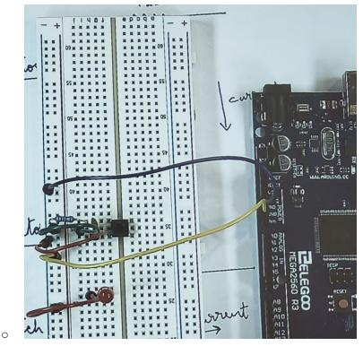
• Connect the 1k Ohm Resistance in series with the LED
